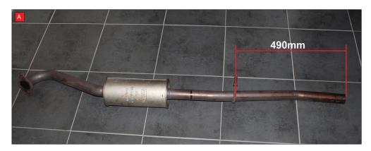
A) To fit the Scorpion rear silencer you will need to cut the O.E centre section. Carefully remove this and accurately measure 490mm from the bracket as shown in figure A and carefully cut the pipe work. Once cut clean and de-bur the cut end. Re-attach the centre section to the car and follow the line diagram on the previous page.
